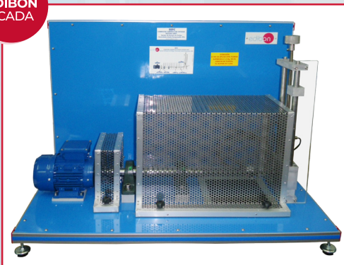
EEFC Computer Controlled Fatigue Testing Unit
