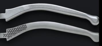
ADAM enables the creation of unique geometries such as closed-cell honeycomb infill. Parts can be printed like the structure of bones - a closed cell inner core encased in a solid outer shell. This geometry is not possible using traditional subtractive manufacturing processes
