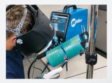
The helmet's heads-up display delivers immediate visual feedback on the user's performance, providing confirmation when parameters are being maintained and alerts when they are exceeded. The same images also appear on the second display panel in the system's computer case.
