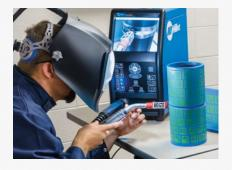
Inside the helmet, the augmented reality environment appears on a specially designed heads-up display panel, precisely showing the user's proximity to and interaction with the workpieces and welding gun/torch. The same images also appear on a second display panel in the system's computer case. Additionally, realistic arc sounds feed through speakers located in the helmet.
