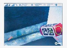
The AugmentedArc system continuously monitors the user's adherence to predetermined or custom welding parameters — including travel speed, gun/ torch angles, distance, aim, contact-tip-to-work (GMAW/FCAW only) and arc length, rod work angle and rod travel angle (GMAW/SMAW).
