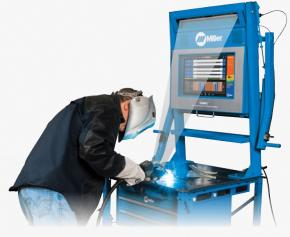
The SmartGun and SmartStinger vibrate whenever predetermined weld parameters are exceeded. This haptic feedback prompts the user to make performance-enhancing adjustments and helps to reinforce optimal gun/stinger positioning and movement.
