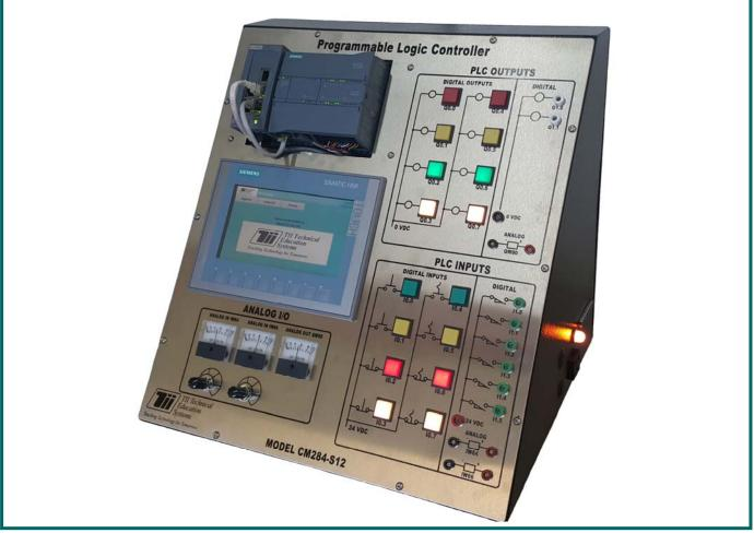
Siemens Integrated Automation Training System Featuring the S7-1200 PLC with Simatic HMI.
