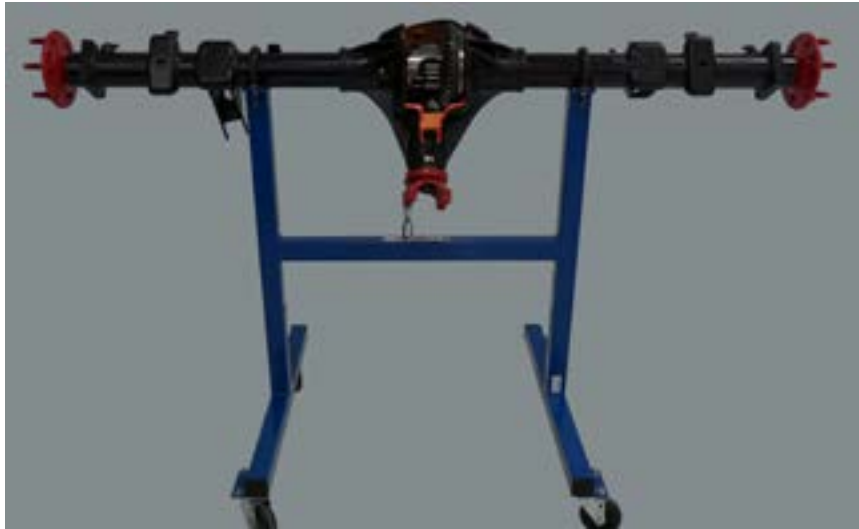
Locking Differential / Limited-Slip Rear Axle Cutaway Model 126
