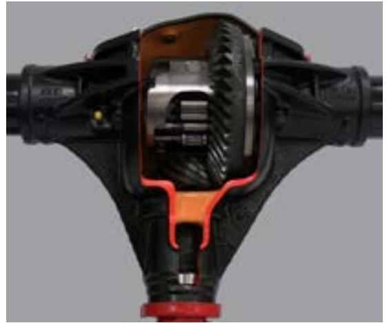
Locking Differential / Limited-Slip Rear Axle Cutaway Model 126
