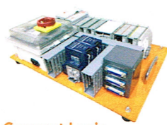
Compact Logix PLC Trainer
