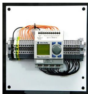
ALLEN BRADLEY PROGRAMMABLE LOGIC MODULE
