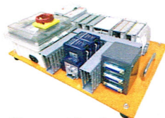
Compact Logix PLC Trainer
