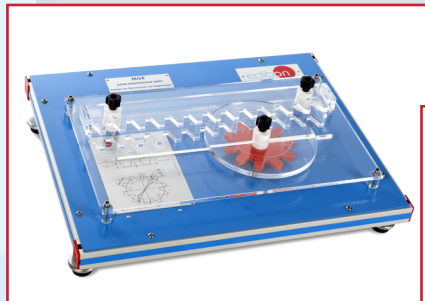
MGE Gear Generation Unit
