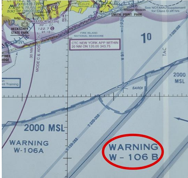
Figure 2.h: Warning areas are often found on the coastline. They are oftentimes identified by blue hatch lines with the word “Warning”, or the letter “W” followed by a dash and a serial number. On the left is an example of what you might see on your sectional chart.
