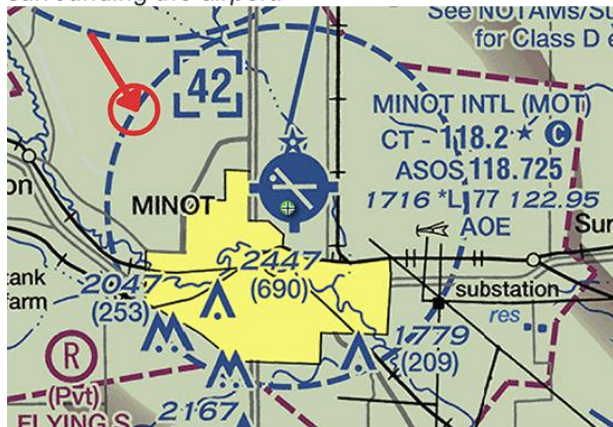
Figure 2.b: To identify Class D airspace, your sectional chart will have blue dashed lines surrounding the airport.
