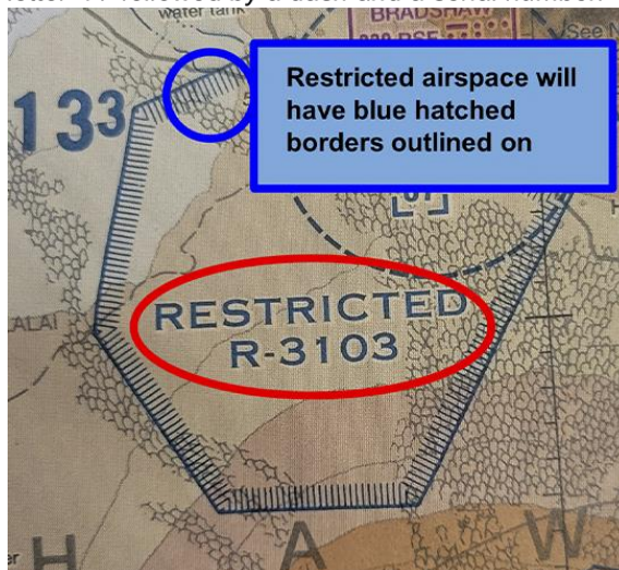
Figure 2.e: Like prohibited areas, restricted areas are identified with a blue hatched border. Inside the border will be the name "Restricted" or the letter "R" followed by a dash and a serial number.
