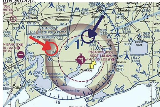
Figure 2.c: To identify Class E airspace on a sectional chart, look for two indicators: a dashed magenta line, which shows the airspace starts at ground level. And a shaded pattern surrounding the airport.
