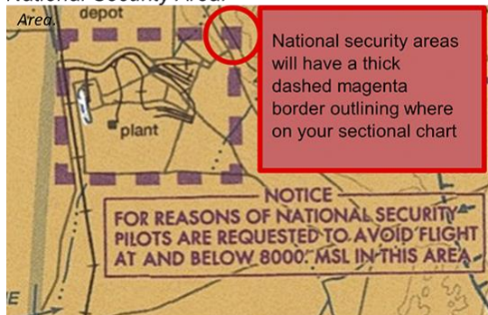
Figure 2.g: National Security Areas (NSA) are identified by thick, dashed magenta lines on your sectional chart. There will also be a notice indicated next to or under the outlined border explaining that the area is categorized as a National Security Area.
