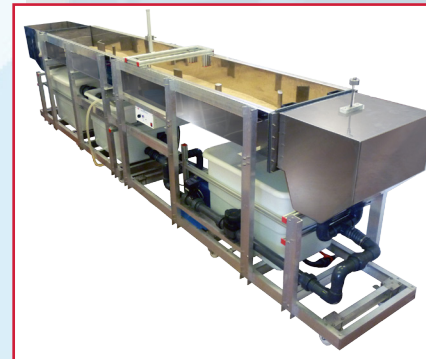
HVFLM-4 Mobile Bed and Flow Visualization Unit (working section: 4000x610 mm)
