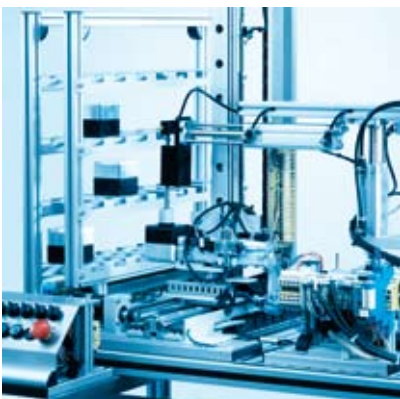
Handling device in front of the high bay racking
